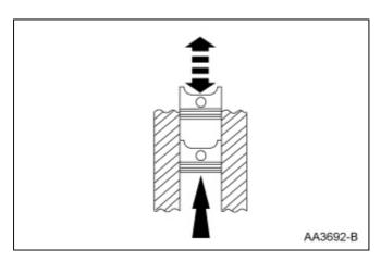
2. Use the Feeler Gauge Set to measure the top piston ring end gap and the second piston ring end gap.
